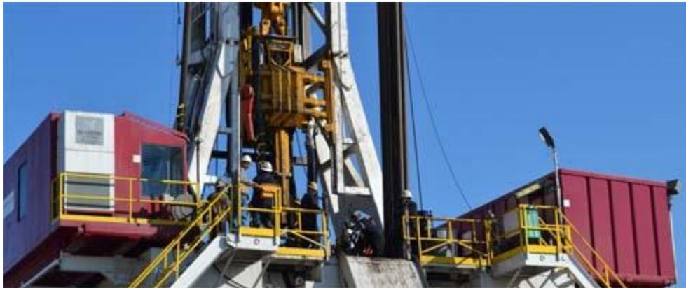
In 2012, Swift Energy began using walking rig technology that enables rigs to be moved from one drilling location to another without having to be dismantled. This reduces rig down time and lowers costs.
