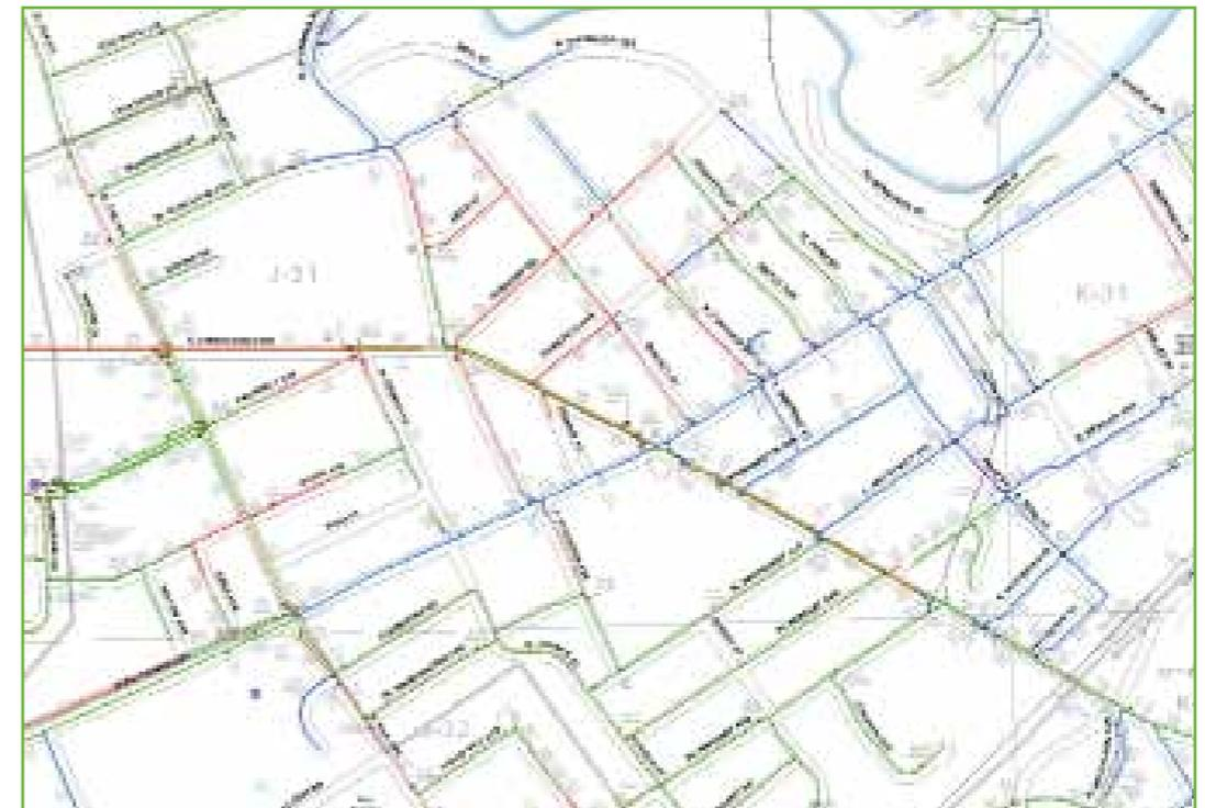
Neighborhood map of the GIS outlining current pipe and valve locations. This system allows workers to quickly locate and identify pipe breaks and leaks while in the field.
